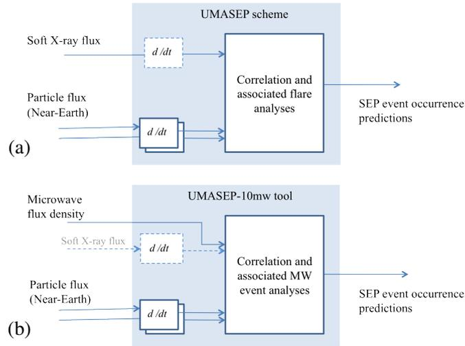
**Fig. 1.** Schematic of the correlation process of the Well-Connected SEP forecasting module of the UMASEP scheme. (a) UMASEP-10, which correlates the time-derivative of soft X-ray flux with the time-derivative of the differential proton fluxes in different energy channels observed by the GOES spacecraft (9-500 MeV). (b) UMASEP-10mw, which uses the microwave flux density instead of the soft X-ray derivative.
