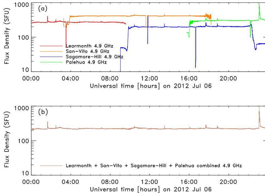
**Fig. 3.** Example of microwave data for a sample 24-hour interval. Panel (a) shows the flux density observed by the four RSTN stations at 4.9 GHz. Spikes, discontinuities, and background are corrected in the combined flux density shown in panel (b).
