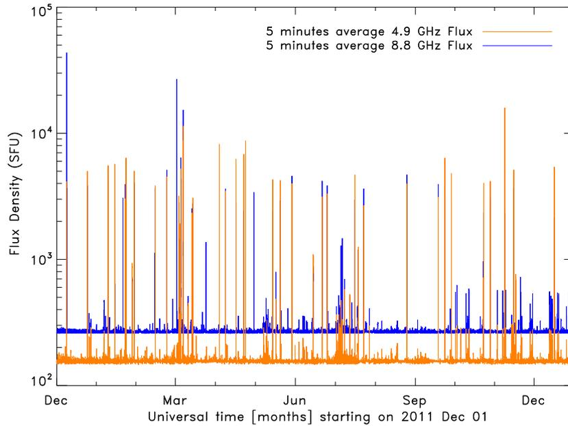
**Fig. 4.** The combined time history of the microwave flux density at two frequencies during the 13 months from 2011 Dec 01 to 2012 Dec 31, constructed from observations of the four RSTN stations. The flux density is averaged over 5 minutes, the background is removed for each instrument, and an average background over the 13 month period is added.
