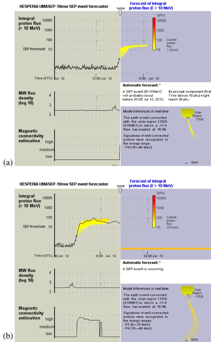
**Fig. 5.** Two UMASEP-10mw outputs after processing microwave data at 5 GHz from 2012 July 12 and GOES proton fluxes of  $> 10$  MeV energies. (a) the prediction at 18:05. (b) the subsequent evolution of the  $> 10$  MeV integral proton flux. The yellow/orange band in the proton intensity plots gives the predicted range, with the colour scale shown by the vertical bar.
