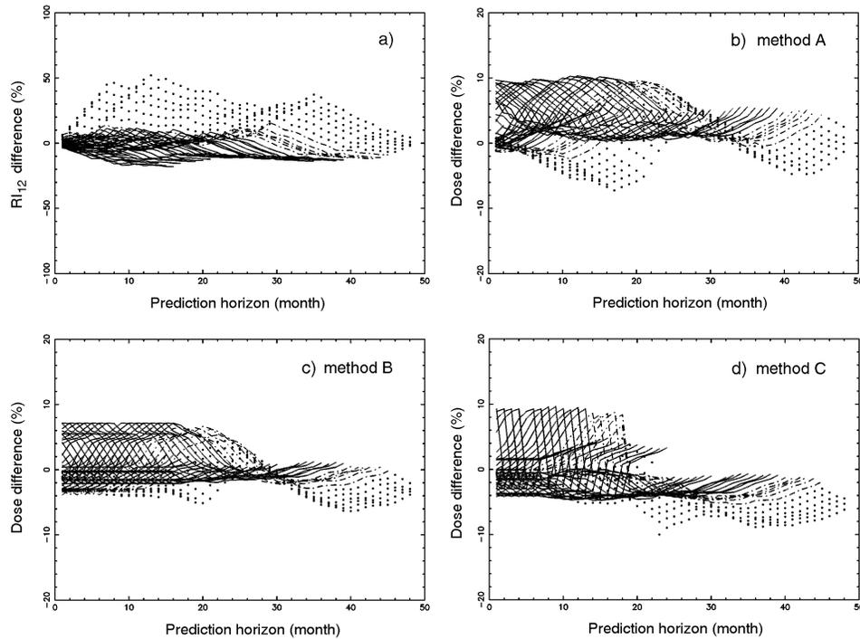
**Figure 6:** Relative errors (in %) of the prediction of  $RI_{12}$  (6a) and of doses received on a Paris- San Francisco flight with methods A (6b), B (6c) and C (6d). The comparison is with variables calculated from 12 month-smoothed cosmic ray observations with Kerguelen NM. See explanations in text.
